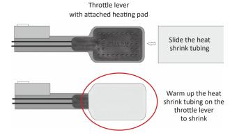
3. Secure the electrical cables to the throttle lever with zip tie, then run the thumb warmer cables along the handlebars and secure them to the handlebars with zip ties. Important: Be sure to leave enough slack in the cables - when moving the throttle lever, the cables must not be stretched to avoid pulling tension.
